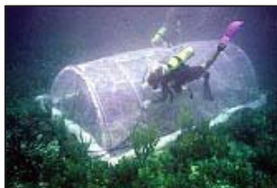
The SHARQ® (Submersible Habitat for Analyzing Reef Quality) experimental chamber is used to measure reef calcification, photosynthesis, respiration, and other process studies of reef communities (contacts: Bob Halley, Kim Yates).
